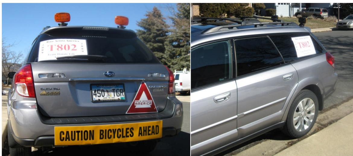
The roof mounted amber flashing lights must be on at all times during the race. The roof mounted amber flashing lights must not be visible from the front. If your lights are the rotating type, the front half must be covered with several layers of tape so as to be not visible to oncoming traffic. It is wise to have extra batteries for those lights.
